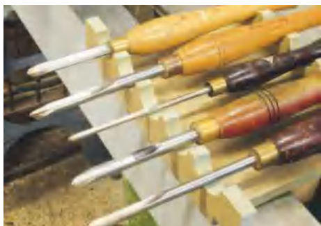
▲ Pic.1 Spindle gouges are available in all sorts of sizes: the far one is a forged tool whereas most modern ones are made from a round bar with a flute milled out
